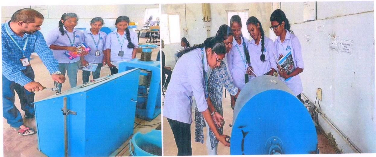
Highway Engineering & Concrete Technology Lab: Testing cube specimen in Compression Testing Machine, Testing aggregates in los angles abrasion testing machine.
